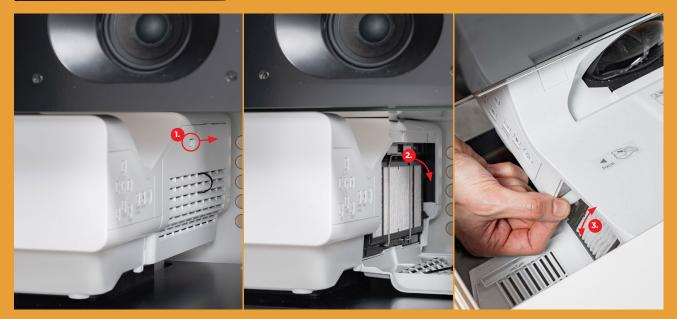
Open the front door by pressing the top left front corner. The image focus adjustment lever is located behind the hatch on the side of the projector. Push the locking mechanism forward (1) to open the hatch (2). Adjust the image resolution from the adjustment lever (3).
